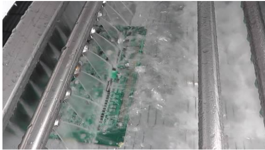
Flood Box Printed Circuit Board traveling through the Flood Box
