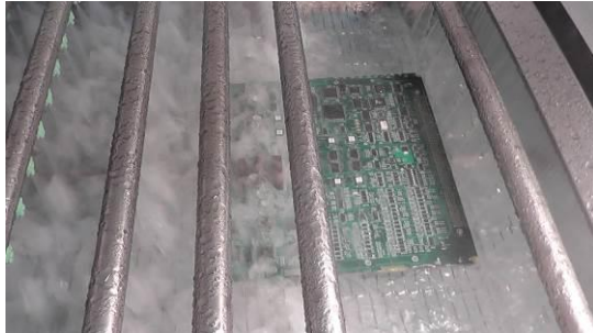
Flood Box Printed Circuit Board completely submerged within the Flood Box
